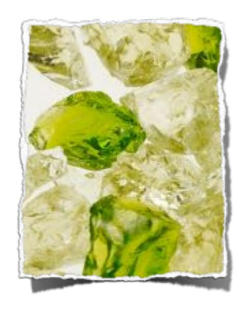
CURAVA quartz slabs are made of polyester resin and quartz, with quartz being the main ingredient by weight.
